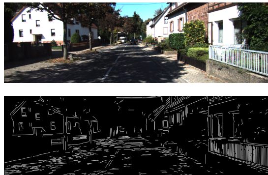
Fig. 2: Image with heavy shadows and edges detected by LSD.
